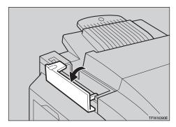
**3** Remove the used oil bottle from the printer carefully.
